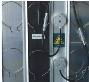
Four sensors monitor UV irradiance
